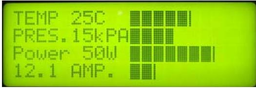
Graph can be drawn from left to right or right to left. The starting point of the graph is the current cursor position. Initialize horizontal graph command ( 0xFE,0x04 ) must be issued before this command can be used. In the example in Figure 15, the starting point of the graph is at column 10.
