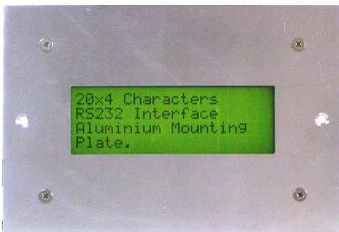
Fig 4. Optional Aluminum Panel Mounting Plate
