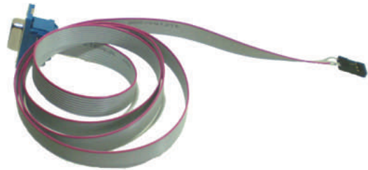
RS232 cable , DB9 Female to P1 Header
