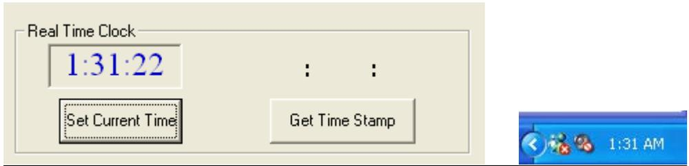
Clicking on the " Set Current Time " button to set up the real time clock using the PC system time.
