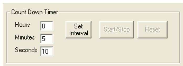
Key in Hours (0-99) ,minutes ( 0-99 ) and seconds value ( 0-59 ). Click on "Set Interval". "Start/Stop" and "Reset" button will be enabled.
