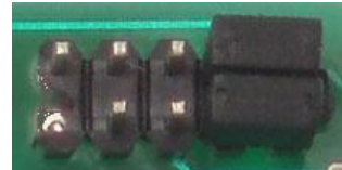
Header P2 ( RS485 Setup )
