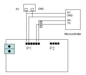
Note: Connection 3 is not required if the inputs and analog ports are not used.
